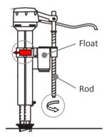
Pull the rod away from the float, as shown. Then, c) adjust the float upwards or downwards, for the desired water level. When complete, d) return the rod into the catch, and twist back 90°; and e) push the red tab back in, to set the float position.
