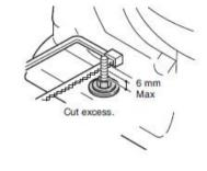
**9)** Connect water supply line, and turn on the water. Flush several times, and check for leaks. Do not overtighten!
